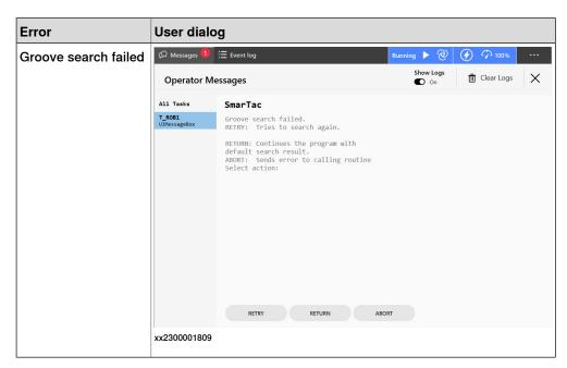
When one of the dialogs above is active, the signal  $doSMT_Dialog_X$  will be high and  $goSMT_Dialog_X$  will be set to 9. The remote device may respond to the dialog by setting  $giSMT_Response_X$  to a value from the list below, followed by pulsing  $diSMT_Ack_X$ .
